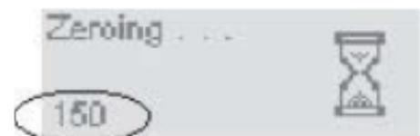
Once the Zero routine is complete the instrument displays its running screen and is ready for use.
