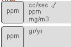
GasCheck Tesla instruments have the capability of displaying detected readings in a variation of units; ppm, cc/s, mg/m<sup>3</sup> and g/yr.
