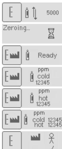
1. Fill an empty (uncontaminated) sample bag with 5000 ppm Helium gas before starting the calibration procedure. Also remove the outer grey probe from the GasCheck G.
