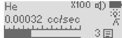
Ensure the instrument is on the X100 (times one hundred) range while on the main running screen. Use the UP and DOWN key to adjust between sensitivity ranges. X100 is most sensitive, X1 is the least sensitive.
