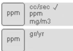
**3** GasCheck G instruments have the capability of displaying detected readings in a variety of units; ppm, cc/sec, mg/m<sup>3</sup> and g/yr.
